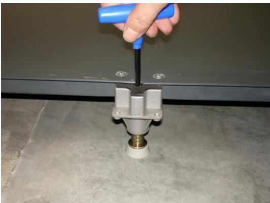
(3) Hexagon key-wrench stretching from top to adjust height
